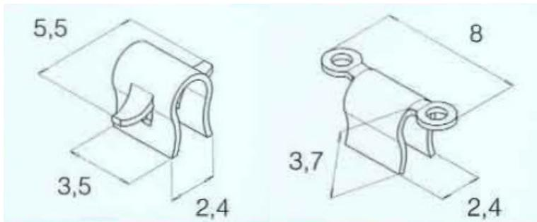
No soldering of the clip. The horizontal retention tangs (**FIG 2-3**) provide firm retention in acrylic and require no additional vertical space. The cylindrical mesial-distal retentions are easily bent to the preferred position prior to processing. There are two different space saving designs.
