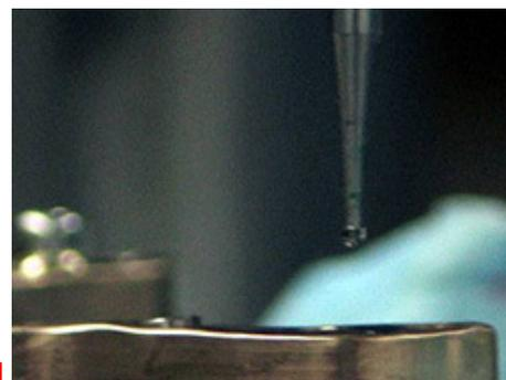
3. Use the 1.7mm Bar Drill (#9102) in a precision drilling device to create the exact size diameter hole to a depth of 2.8mm that is needed for tapping the site (**FIG 2**).
