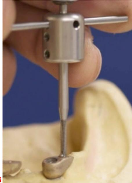
The use of tapping fluid while cutting the threads is required to reduce the chance of breaking the tap off in the preparation. A light lubricant also helps carry metal shavings out of the recess. (**FIG 4-5**). If a tap begins to bind, back the tap out to remove metal shavings. If the shavings are not removed by reversing the tap, you risk breaking the tap.
